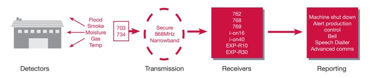
By connecting third party environmental monitoring equipment into 762 or 768 radio transmitters, a radio based facilities monitoring solution can be
